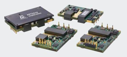
ADQ500 series quarter-brick isolated DC-DC converters produce a single fully regulated 12 V output. Rated at 500 watts, these converters can deliver up to 42 amps output current and have no minimum load requirement. They have an input voltage range of 36 to 75 V and are primarily designed for use with standard 48 V supplies in computing and server applications, as well as regulated 48V supplies in communications equipment.
