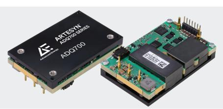
ADQ700 series quarter-brick isolated DC-DC converters produce a single fully regulated 12 V output. Rated at 700 watts, these converters can deliver up to 58 amps output current and have no minimum load requirement. They have an input voltage range of 40 to 60 V and are primarily designed for use with standard 48 V supplies in computing and server applications, as well as regulated 48V supplies in communications equipment.
