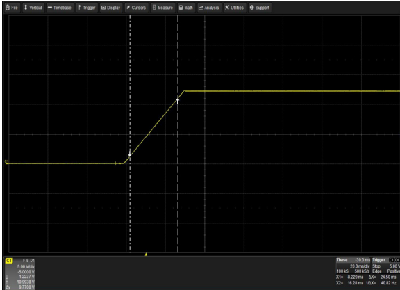
Figure 19: CSU2000AP-3-111 Output Voltage Startup Characteristic Vin = 90Vac Load: Io = 102.5A I SB = 3.5A Ch 1: V O
