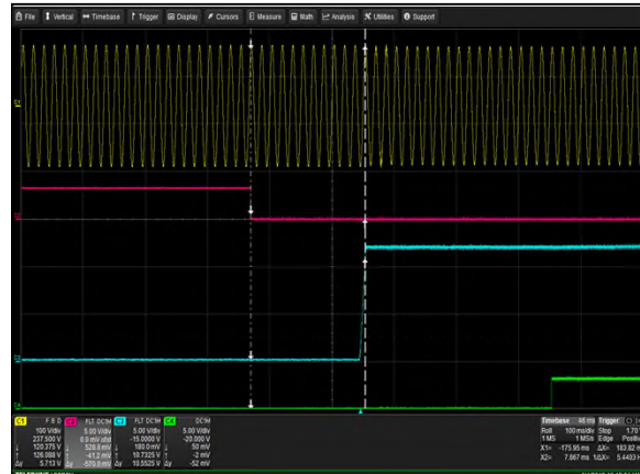
Figure 2: DS2400SPE-3 Turn-on delay via PSON - Vin = 90Vac Full Load: I_o = 114.75A , I_{SB} = 3.5A , Turn-on delay: 183.82ms Ch 1: AC Mains Ch 2: PSON Ch 3: V_o Ch 4: PWR_GOOD (PWOK)
