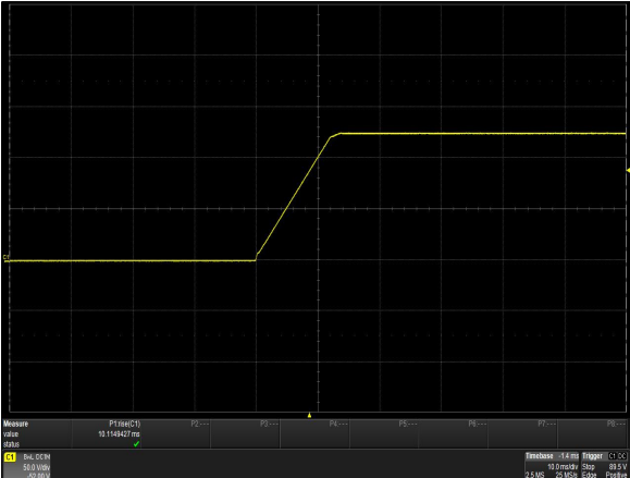
Figure 27: iHP24H3A-S1-00 Output Voltage Startup Characteristic Load: I_o = 12A Ch 1: V_o
