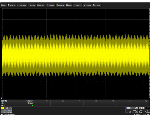
Figure 11: LCC1200-28U-9P Ripple and Noise Measurement Vin = 230Vac Load: Io = 42.9A (28V), I SB = 1.5A (5V) Ch 1: V O
