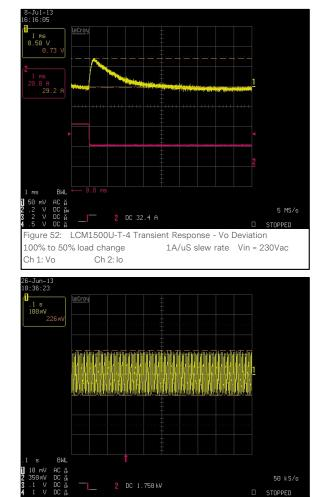
Figure 54: LCM1500U-T-4 Ripple and Noise Measurement Vin = 115Vac Load: Io = 42A (36V), Isb = 2A (5V) Ch 1: Vo
