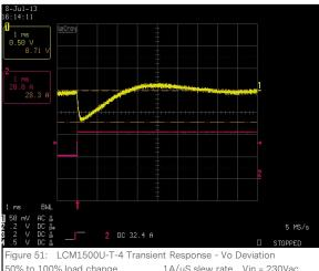
50% to 100% load change 1A/uS slew rate Vin = 230Vac Ch 1: Vo Ch 2: lo
