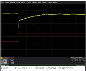
50% to 100% load change 1A/uS slew rate Vin = 230Vac Ch 1: Vo Ch 2: lo
