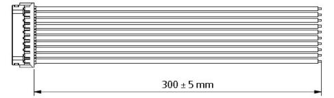
2. Order kit part number 73-788-002 for control connector interface with unloaded housing and 20 pins
