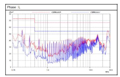
The LCM1500 series have internal EMI filters to ensure the convertors' conducted EMI levels comply with EN55022 (FCC Part 15) Class A.
