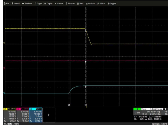
Figure 12: PS1650 Turn Off Characteristic via PSKill V_{IN} = 180\text{Vac} , I_O = 67.35\text{A} Ch 1: V_O Ch 2: PSU_Alert# Ch 3: PSKill
