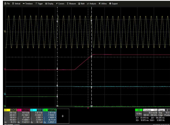
Figure 6: PS1650 Turn-on delay via PS_ON# – V_{IN} = 180\text{Vac} Full Load: I_O = 134.7\text{A} Ch 1: AC Mains Ch 2: V_O Ch 3: PSU_Alert# Ch 4: PS_ON#
