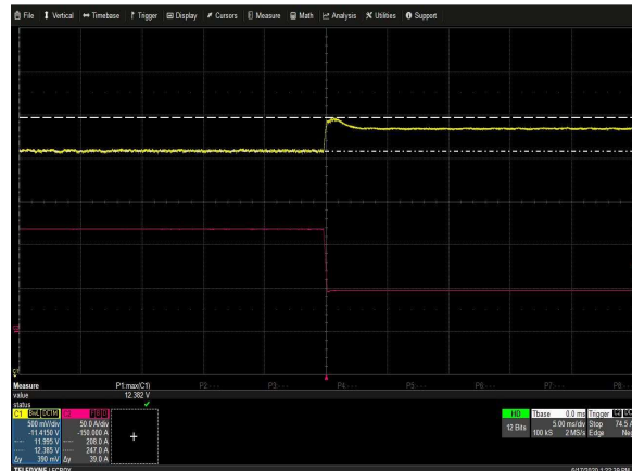
Figure 14: PS1650 Transient Response – V_O Deviation (high to low) 40% to 100% load change, 0.25\mu\text{s} slew rate, V_{IN} = 230\text{Vac} Ch 1: V_O Ch 2: I_O
