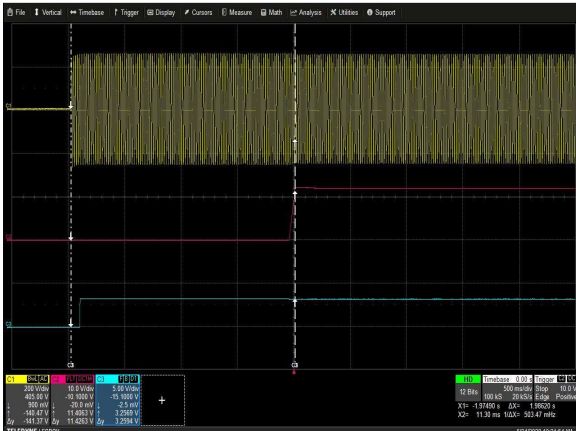
Figure 5: PS1650 Turn-on delay via AC mains – V_{IN} = 180\text{Vac} Full Load: I_O = 134.7\text{A} Ch 1: AC Mains Ch 2: V_O Ch 3: PSU_Alert#
