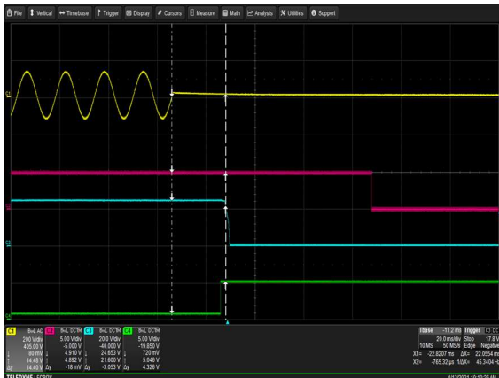
Figure 21: μMP10T-S2Q-S2Q-S2Q-S2Q-S2Q-S2Q-90-A Hold-up Time via AC mains Vin = 90Vac/63Hz Load: I O = 41.66A I SB = 2A Ch 1: AC Mains Ch 2: V SB Ch 3: V O Ch 4: Global DCOK
