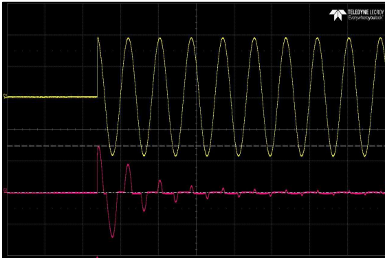
Figure 7: μMP04T-S2P-S2P-S2P-60-A Start up Inrush Current Vin = 264Vac Load: I O = 0A I SB = 0A Turn On Phase = 90° Ch 1: V IN Ch 2: I IN
