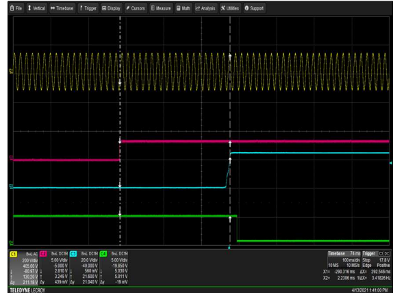
Figure 20: μMP10T-S2Q-S2Q-S2Q-S2Q-S2Q-S2Q-90-A Turn-on delay via Global inhibit Vin = 90Vac Load: I O = 41.66A I SB = 2A Ch 1: AC Mains Ch 2: Global inhibit Ch 3: V O Ch 4: Global DCOK
