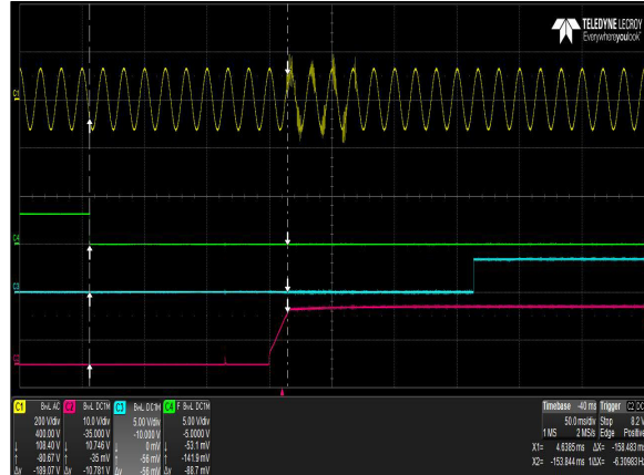
Figure 2: DS1200HE-3-002 Turn-on delay via PS_ON – Vin = 90Vac Full Load: Io = 83.3A, Isb = 4A (5V) Ch 1: AC Mains Ch 2: Vo Ch 3: POWER GOOD Ch 4: PS_ON
