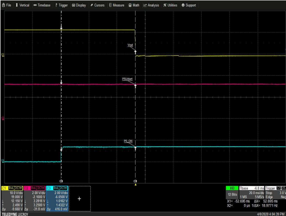
Figure 22: PS1000 Turn Off Characteristic via PS_ON Full Load: I_o = 80A Ch 1: PS_ON Ch 2: V_o Ch 3: PSU_Alert
