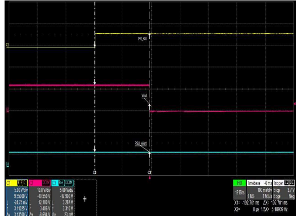
Figure 12: PL1000 Turn Off Characteristic via PS_Kill Full Load: I_o = 80A Ch 1: PS_Kill Ch 2: V_o Ch 3: PSU_Alert
