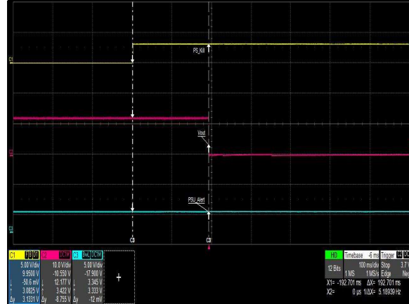
Figure 23: PS1000 Turn Off Characteristic via PS_Kill Full Load: I_o = 80A Ch 1: PS_INHIBIT Ch 2: V_o Ch 3: PSU_Alert
