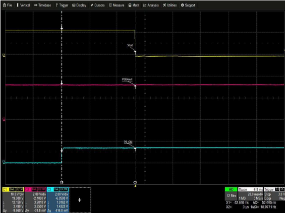
Figure 11: PL1000 Turn Off Characteristic via PS_ON Full Load: I_o = 80A Ch 1: V_o Ch 2: PSU_Alert Ch 3: PS_ON
