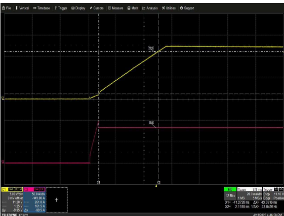
Figure 20: PS1000 Output Voltage Startup Characteristic – V_{IN} = 180Vac Full Load: I_O = 80A Ch 1: V_O Ch 2: I_O
