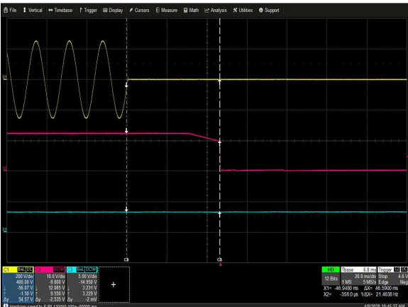
Figure 18: PS1000 Hold-up Time – V_{IN} = 90Vac / 60Hz / 0^\circ Full Load: I_O = 80A Ch 1: AC Mains Ch 2: V_O Ch 3: PSU_Alert
