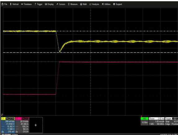
Figure 24: PS1000 Transient Response – V_o Deviation (low to high) 40% to 100% load change, 0.2A/\mu S slew rate, V_{IN} = 230Vac Ch 1: V_o Ch 2: I_o
