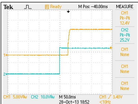
Figure 47: AEE00BB24-M Output Voltage Startup Characteristic by Vin Vin = 24Vdc Load: Io = ±0.417A Ch1: Vo1 Ch2: Vin
