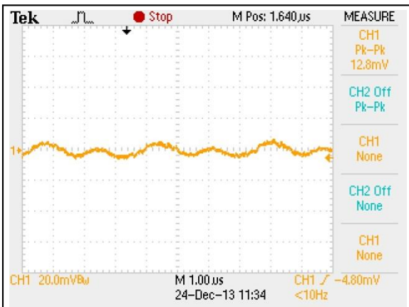
Figure 48: AEE10F36-L Ripple and Noise Measurement Vin = 24Vdc Load: Io = 10A Ch 1: Vo
