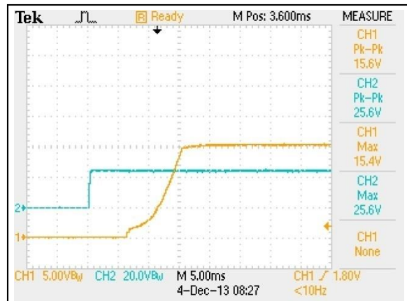
Figure 33: AEE03C18-L Output Voltage Startup Characteristic by Vin Vin = 24Vdc Load: Io = 3.33A Ch1: Vo Ch2: Vin
