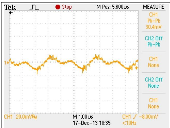
Figure 75: AEE03C36-L Ripple and Noise Measurement Vin = 48Vdc Load: Io = 3.33A Ch 1: Vo
