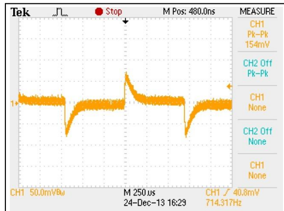
Figure 76: AEE03C36-L Transient Response Vin = 48Vdc Load: Io = 100% to 75% load change Ch 1: Vo
