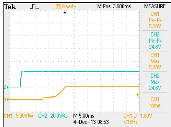
Figure 15: AEE10A18-L Output Voltage Startup Characteristic by Vin Vin = 24Vdc Load: Io = 10A Ch1: Vo Ch2: Vin
