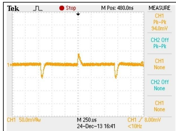
Figure 4: AEE10F18-L Transient Response Vin = 24Vdc Load: Io = 100% to 75% load change Ch 1: Vo
